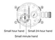
If the small hour and minute hands, and the small 24-hour hand are not at 12 o'clock, rotate the crown to align them with 12 o'clock.
