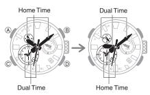
If a swapping operation causes a change in the day indicator setting, the mode hand will rotate repeatedly.
